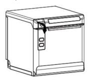
2) In the correct direction of the roll paper, insert the paper.
