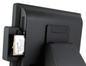
Slide in/out HDD Replacement
