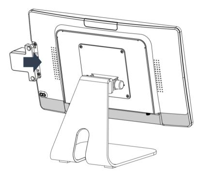
**5.** Secure the barcode scanner with the included two M3x6 screws to the touch computer.
