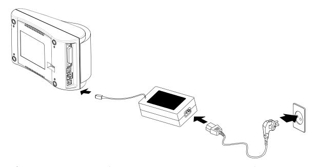
2-1-4 Connect the power cord of the AD adapter to the power terminal of the printer.
